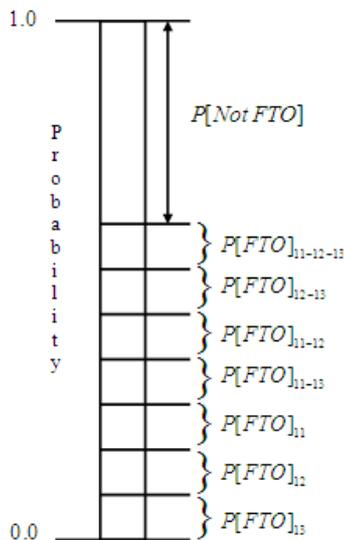
Fig. 7. Sample space for failures to open at circuit breakers
