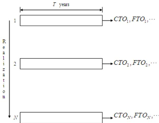
Fig. 3. General procedure of the reliability assessment algorithm
