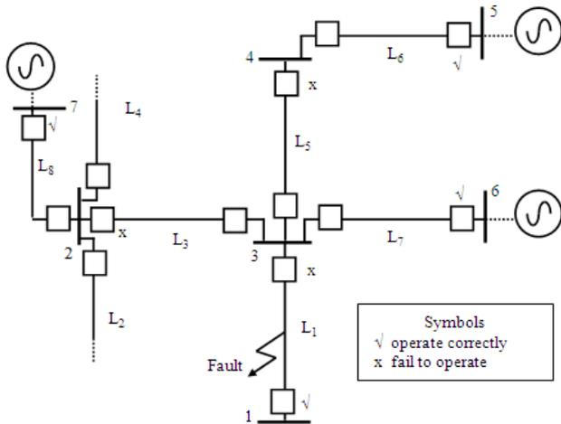
Fig. 1. Analysis on the effect of protective system failures to open
