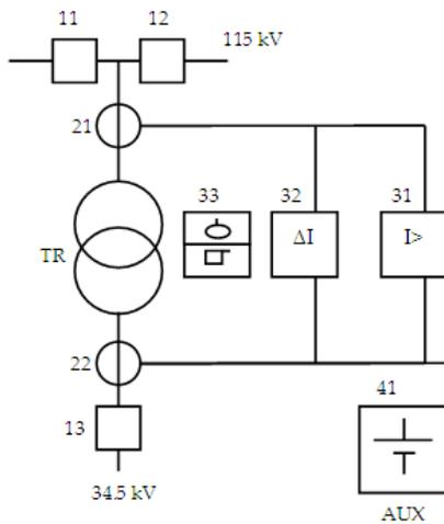
Fig. 5. Protective system of a power transformer
