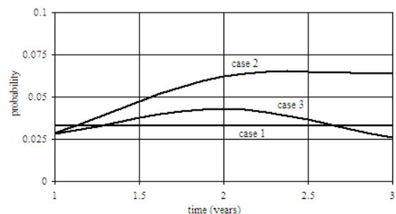
Fig. 6. Probability of failure to open at circuit breaker 13
