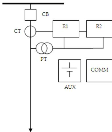
Fig. 2. Protective system at a terminal of a transmission line
